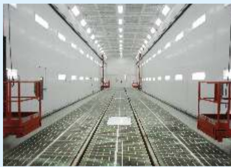
Air exhausted by pits
