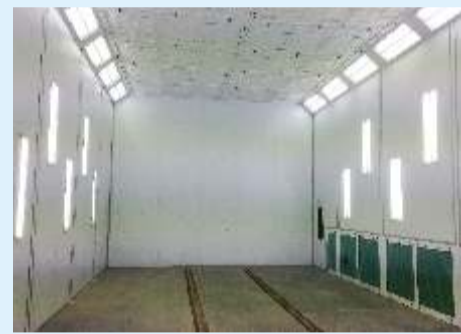
Air exhausted by single side wall
