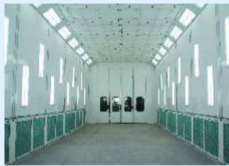
Air exhausted by two side walls
